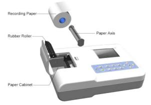
Figure 6-1 Installation of recording paper
